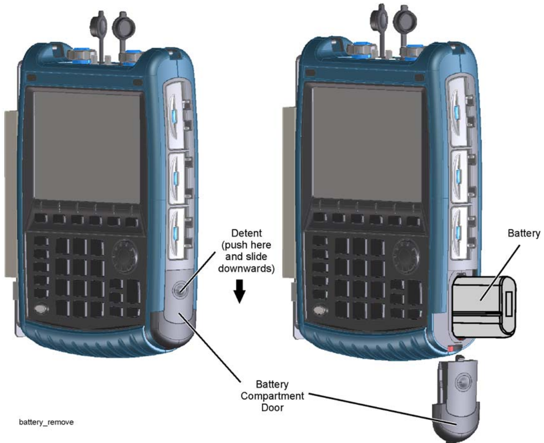
Figure 7-1 Replacing the Main Battery
